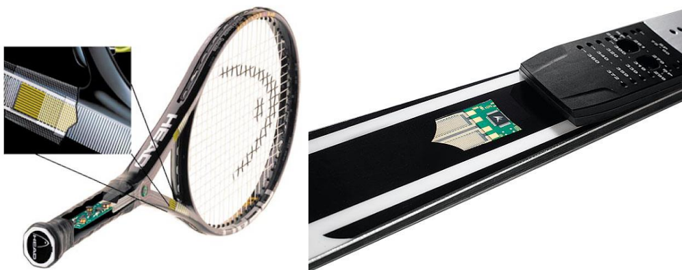
Figure 10: AFCs & electronics may be integrated into tennis rackets (left) and also embedded in sandwich construction of alpine skis (right).
